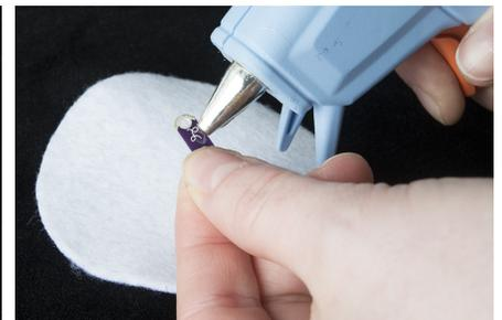
not on top of the battery holder. Make sure the + and - symbols line up with the symbols on the battery holder. Be careful not to cover the holes with glue - we'll need those to sew through later. *Do not put your battery in yet.*
