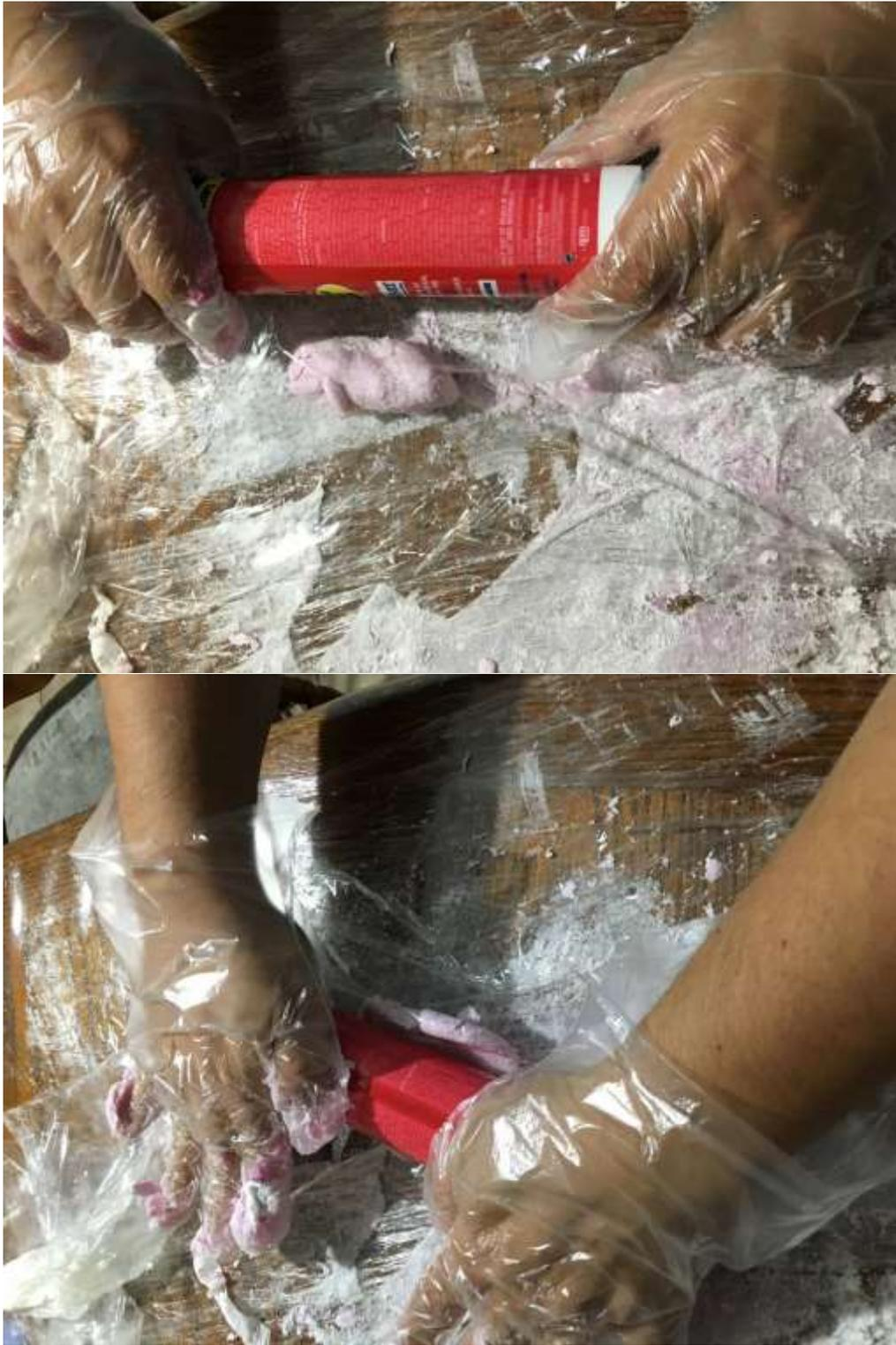
*Figure 10: Rolling the silicone/starch mixture*
