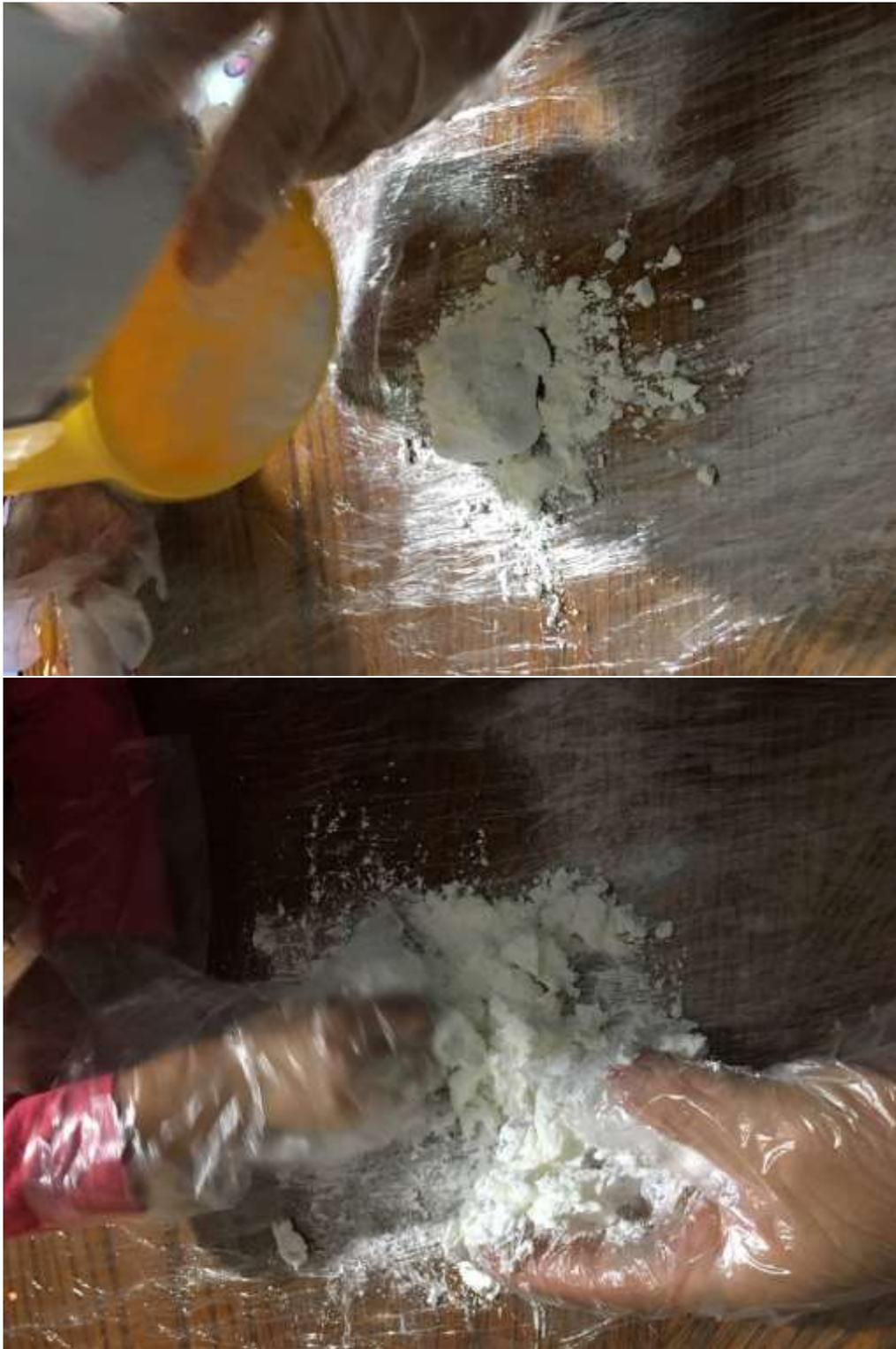
*Figure 7: Mixing starch with silicone on the workstation*
