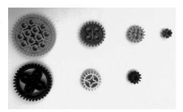
where X is less than Y. Note that X equals the number of teeth on the output gear and Y equals the number of teeth on the input gear.
