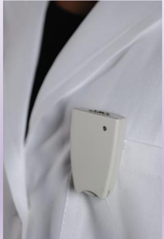
Pocket dosimeter; a NMR monitoring device with three Hall-effect sensors 2010 Elia.braggio , Wikimedia Commons (public domain) https://commons.wikimedia.org/wiki/File:Pocket_Dosimeter.jpg
